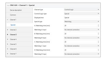
Each channel supports up to 4 functions to monitor the transmission frequency of EnOcean devices:
