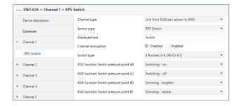
The configuration of a 4-fold rocker is analogous to the 2-fold rocker (F6-02-01), however, it must be noted that for the complete integration, 2 channels must be used in the gateway, one channel for rockers A-B, another channel for rockers C-D. When using a 4-fold rocker, channel encryption is not supported.
