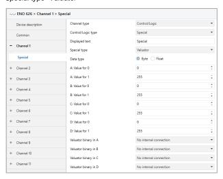
Each channel supports up to 4 valuators to output byte values, or up to 2 valuators to output 2-byte float values:
