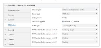
Each pressure point of the 2 rockers can be individually assigned to KNX functions by the parameters "KNX function Switch pressure point":
