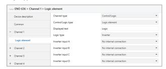
Each gate channel supports up to 4 separate inverters:
