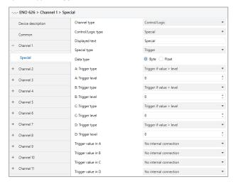
Each channel supports up to 4 triggers for evaluation of byte values, or up to 2 triggers for evaluation of 2-byte float values:
