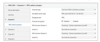
With this profile, a complete RPS switch with 2 rockers can be emulated. Each rocker is separately configurable, the following functions are available:
