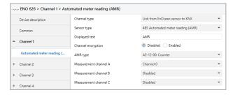
A maximum of three counter channels are supported for each channel. The counter channels that the EnOcean device transmits must be known and set in the parameter. Two communication objects are available for each counter channel, one for the current consumption and for the total consumption.
