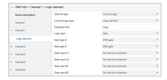
Each gate channel has 2 gates with individually configurable type:
