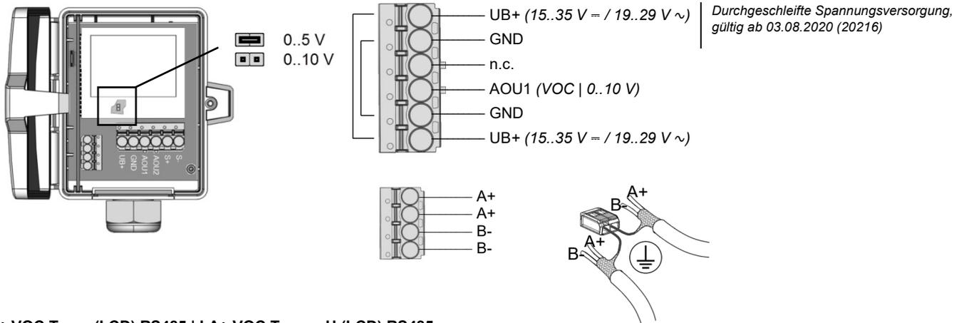
LA+ VOC Temp (LCD) RS485 | LA+ VOC Temp\_rH (LCD) RS485
