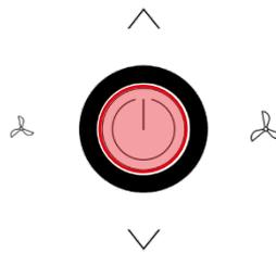
\*If the key is used as a presence key at the same time, the key must be pressed for at least 3s, in all other cases a short press is sufficient.
